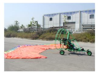
5. Make sure that the trike is placed close to the center of the trailing edge.
