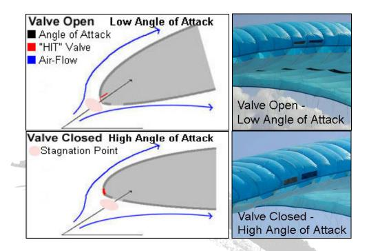
The NRG is equipped with an Active HIT Valve system (patent pending) to improve the overall performance and safety of the wing especially during accelerated flight.
