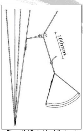
Figure 16-1 Brake Line Adjustment
