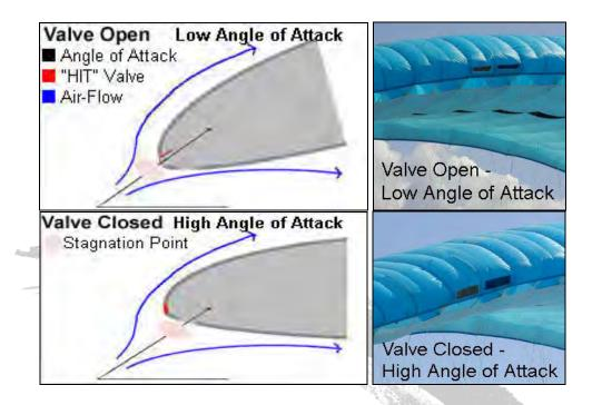
The FORCE is equipped with an Active HIT Valve system (patent pending) to improve the overall performance and safety of the wing especially during accelerated flight.
