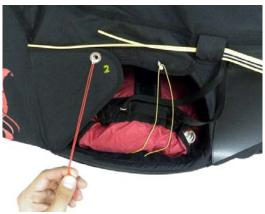
7. Now close flap No.1 over the reserve and thread the first pull cord through the grommet on flap No.2.
