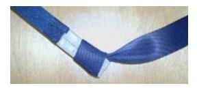
3. Attach the reserve parachute bridle to the center of the harness bridle using a larks head knot, sealed with a heat shrink tube to keep it in place as shown.
