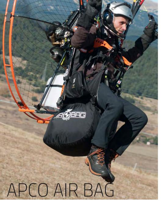
or about 70 €, the manufacturer Apco offers an airbag which can, as an option, attach under the Split Legs harnesses. The airbag quickly takes shape when flying; its volume seems substantial and, its ability to shock absorb should be correct, or even pretty good (there are no official measurements). Obviously an Airbag of this size will slightly increase the drag on a paramotor, but the safety for the pilot is worth it!
