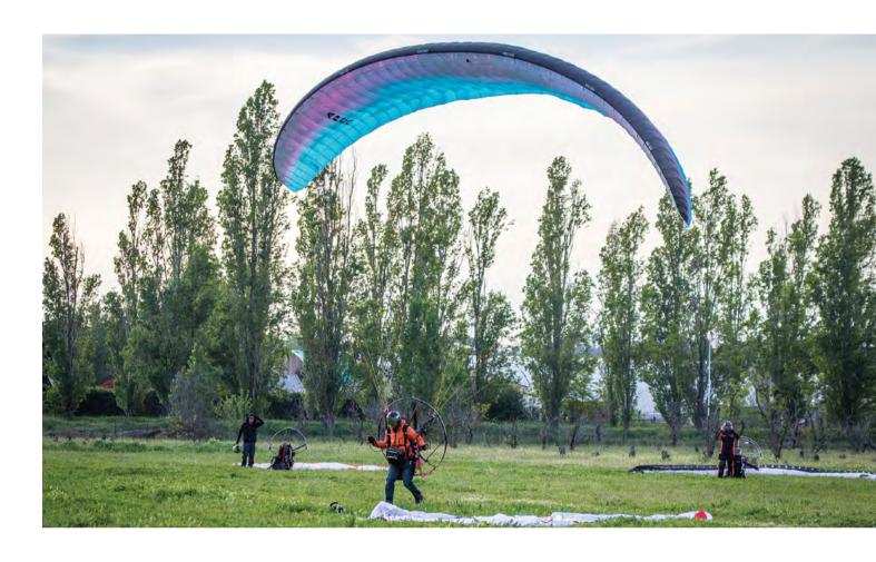
In stronger winds the wing is equally easy to use. Again a firm pull on the wing will get it climbing steadily above your head. Moving under the wing as it comes up keeps everything calm and you can feel the lift being generated. This means very few steps are needed before you are in the air.
